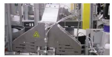
The Mespack UHS top sealer is a continous sealing system. It is specially designed to avoid film burn in the event case of machine stops.
