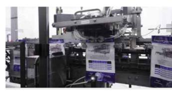
Our infeed conveyor system includes a 3-phase motor for The pouch opening system includes Pneumatic actuators and destacker and flapper wheels and three photoelectric sensors to vacuum cups to ensure a good aperture before the filling station.
