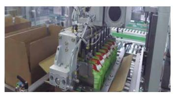
After the grouping and picking process, all the pouches are introduced into the box at once.
