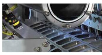
Our unique pouch detector vision system checks for proper film forming in drum cavities. If there is no detected film, no fill takes place. This feature saves you valuable time, by preventing unnecessary clean-ups.
