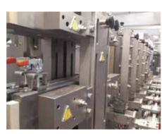
A quick changeover reduces material waste when the format is changed. The preparation of a pouch format change requires not only time, but also film and energy consumption. Both automatic and mechanic quick changeovers will reduce time, film, and energy. It is a tool-free and user-friendly operation.
