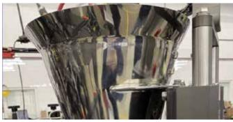
This quick changeover tool-less system for funnels and baffles is design to enhance format change time.
