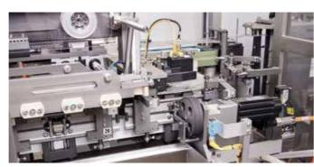
CMR's automatic quick changeover system allows for a quick width change from one format to another.
