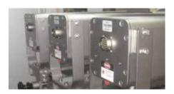
The printing or coding area of the MS Series is integrated into the machine unwinder, thus additional protection is unnecessary. Moreover, the support for this area is independent, in order to avoid the possibility of vibrations.
