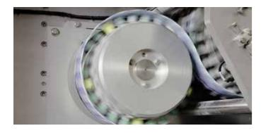
The Mespack UHS rotary cutting system is servo driven and controlled by HMI. It helps to increase the line efficiency.
