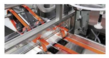
Our infeed conveyor is able to work with different pouch types, such as flat pouches, stand-up pouches, box pouches, zipper or corner cap pouches, etc. Up to 4 rails.
