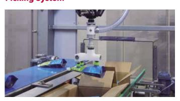
A delta robot is used to pick pouches and place them inside of american box in a horizontal position. Up to 160 picks per minute are possible with a model MCP4.
