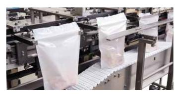
A conveyor belt to support the space surrounding the filling area, which is specially designed for heavy pouches or products that are difficult to dose. The vibration system is also integrated into this component.
