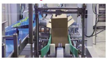
This belt is able to do an american box format change over through HMI in less than the 30s thanks to its full servo characteristic.
