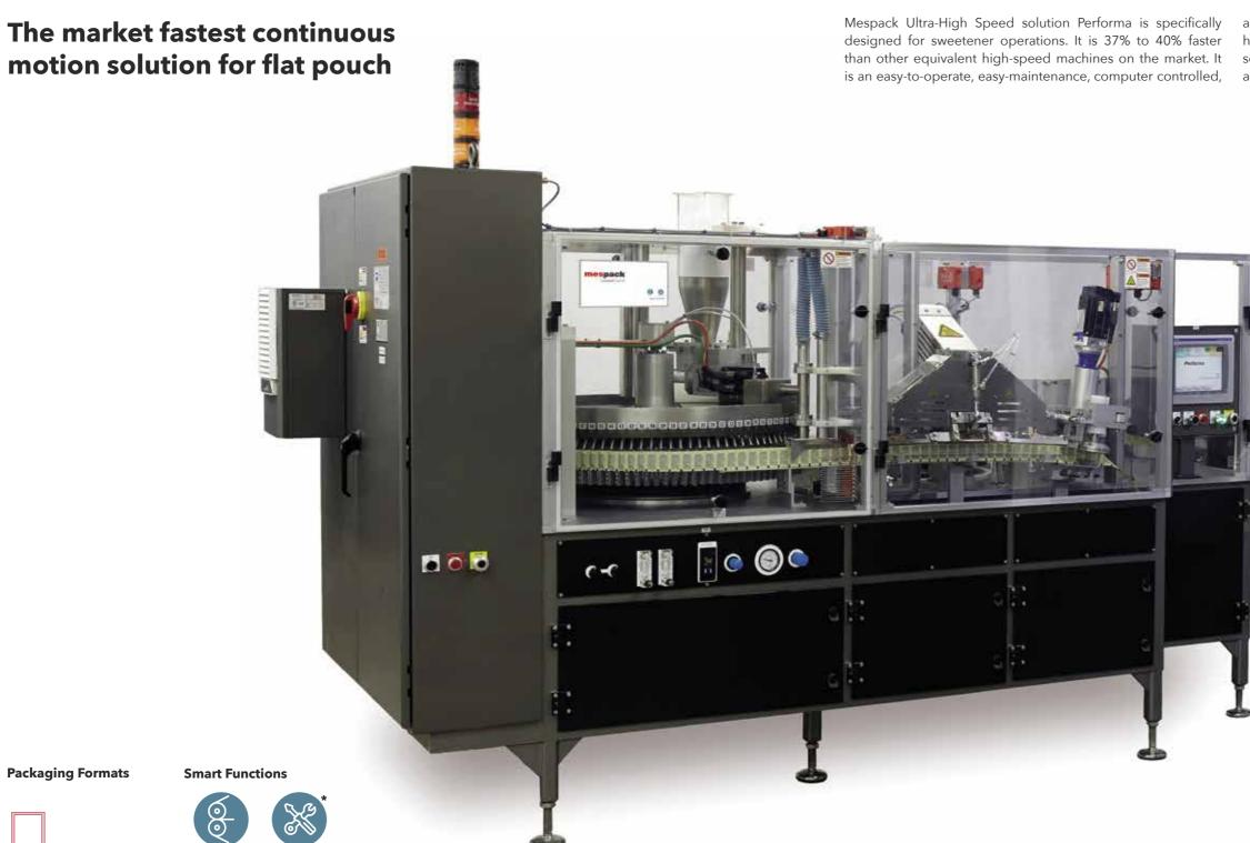
all-servo drive pouch packaging system for high speed and high-volume, with continuous motion horizontal form, fill and seal applications. It is designed for exact count collations and achieves ultra-accurate fills.
