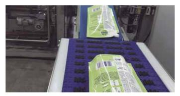
This belt speeds up to change the distance between two pouches from the previous station in order to be adapted to the picking speed.
