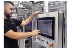
In harmony with its straightforward usability, this series of machines continues to use the Athena platform, with which the operator can monitor, at all times, the OEE ratio as well as that of rejected pouches, among others.
