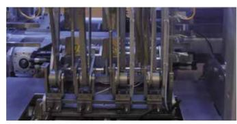
The knives are constructed from special thermally treated steel, which increases durability. Furthermore, the changeover can be performed without tools.
