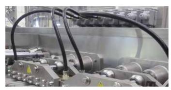
Three set of sealing jaws are available for top sealing and cooling. The pressure control of the top jaws is separate for each jaw. Independent adjustments can be configured on the touch screen.
