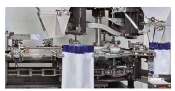
The IMP Series can operate with packages that contain as little as a few ounces to greater than 12 pounds. The impressive filling options include: multi-head weighing, augers, cup fillers and manual. Customers are also able to perform a combination of automatic and manual fillings.
