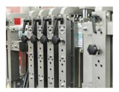
Our experience in flexible packaging has allowed us to offer a quick changeover system for sealers, which reduces the adjustment time. Furthermore, our sealing groups are able to work with various materials, thus obtaining optimum quality with minimum energy consumption.
