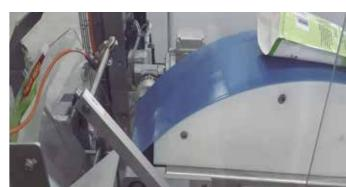
This system allows pouches or other containers to be properly aligned for the next packaging step.
