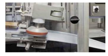
This is the second film drive. It functions as the finishing top seal while the film is being pulled.
