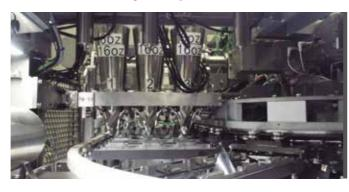
The Mespack mechanical carrousel system offers the possibility of using intermittent or continous motions to discharge. Moreover, due to its grippers management system, extra volume can be used with a higher speed.
