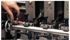
Quick changeovers reduce time and material waste when the format is changed.
