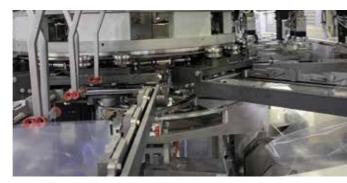
The Mespack triple pouch opening system can perform an aperture of three pouches at the same time with a unique actuator.
