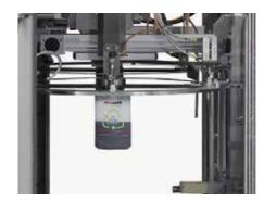
The star system not only operates as separator for the stream of pouches, but it is also used for code printing and visual inspection with in-place pouch rejection.
