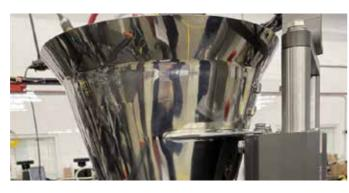
This quick changeover tool-less system for funnels and baffles is designed to enhance format change time.
