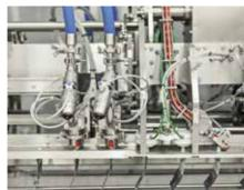
The continuous dosing system is equipped with a hygienic nozzle design. Additionally, a special in-line spout cleaning system, which sprays filtered water, ensures the removal of residual product on the spout or pouch.
