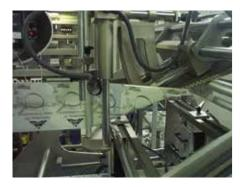
The forming triangle helps fold the film in order to obtain the desired pouch form for both flat pouches as well as stand-up pouches.
