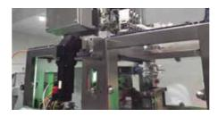
This machine is made of stainless steel in order to operate with pharmaceutical products. The full servo motorized system is also implemented into it, this gives you more coordinating control of the equipment movements.
