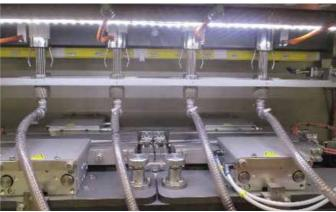
The Clean In Place process allows you to clean the filling circuit with disassembling the filler system, it is based on flushing hot water and chemical solutions through the equipment pipes that have direct contact with the products. its physical, chemical and bacterial action removes dirt and neutralizes surface microorganisms.
