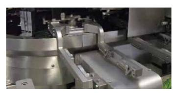
The gripper width for all sealing jaws is adjustable from the HMI via the Mespack Grippers Management System (MGMS). Auto-positioning of all the machine's rear grippers allows for perfect clearance of the filling area, as well as adequate cleaning and sanitizing.
