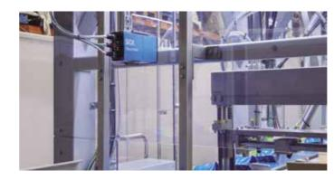
The vision system is integrated into the machine entry. It is used to detect pouch position in order to transmit it to the picking robot.
