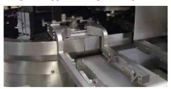
The gripper width for all sealing jaws is adjustable from the HMI via the Mespack Grippers Management System (MGMS). Autopositioning of all the machines rear grippers allow the filling area to be perfectly cleared, as well as adequately cleaned and sanitized.
