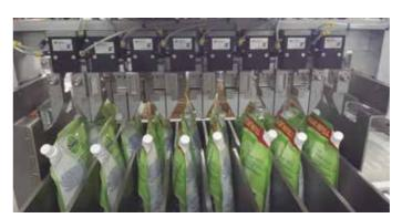
This system works with different patterns, it is specially designed to pick pouches from the indexing system and place them in the correct position in order to be introduced.
