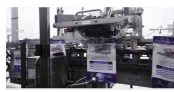
The pouch opening system includes pneumatic actuators and vacuum cups to ensure that there is an optimal aperture before the filling station.
