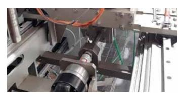
The automatic quick changeover is controlled by servo and can easily be performed by HMI. Furthermore, it avoids operator errors during the changeover process.
