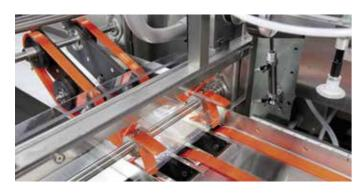
Our infeed conveyor system includes a 3-phase motor for destacker and flapper wheels and three photoelectric sensors to secure the position when tranfer into the machine occurs.
