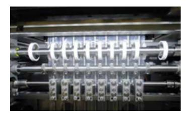
Servo motor is integrated into the film transport system in order to control and correct its position. This system has more operational precision, and gives you more coordinating control of the equipment's movements.
