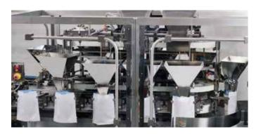
Our traveling funnel is used for such a continuous as an intermittent motion machines. This system significantly increases the speed of the machine.
