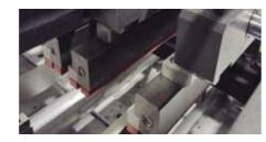
It is a servo-driven unit with blades that move up and down. This makes them a safe cutting system and facilitates the separation of the strings into individual pods.
